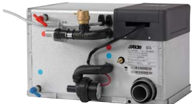
Customer-adapted model with pre-assembled circulation pump, automatic bleeding and fresh water connections.
